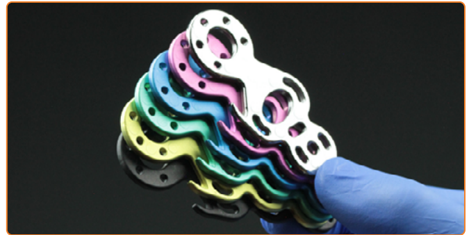
Figure 26 | Different colours made by anodizing titanium MIM parts
