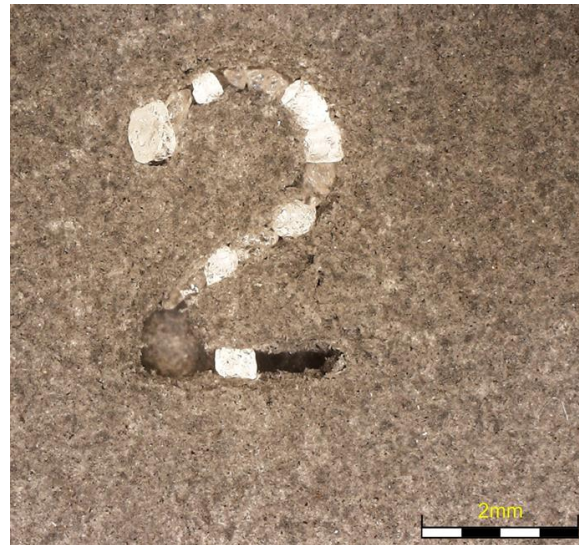
Figure 3. Blasting media incrustated into a part engraving
