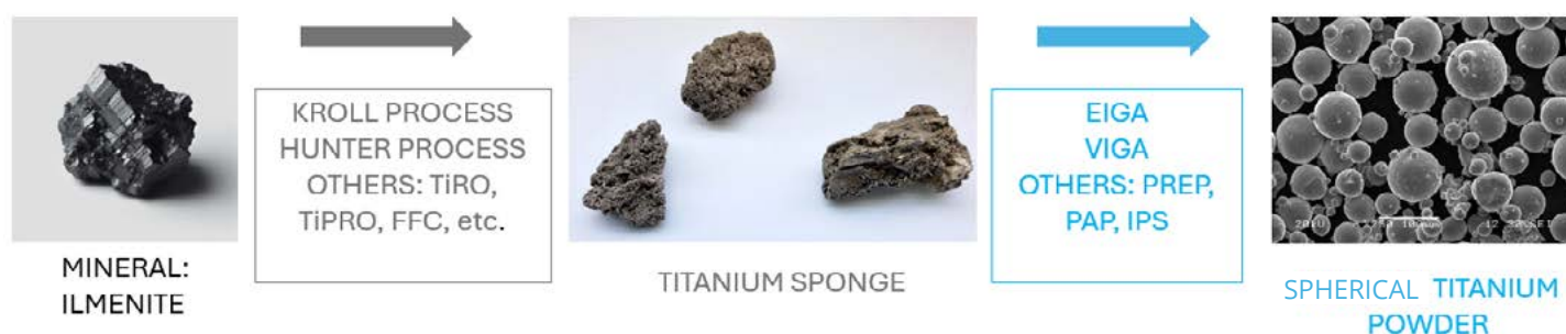
Figure 7 Conventional routes for the fabrication of titanium spherical powders
